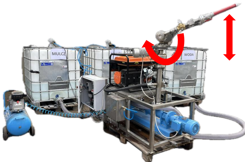
Fig. 4. Automated spraying system under test, with indicated spray cannon operating directions
