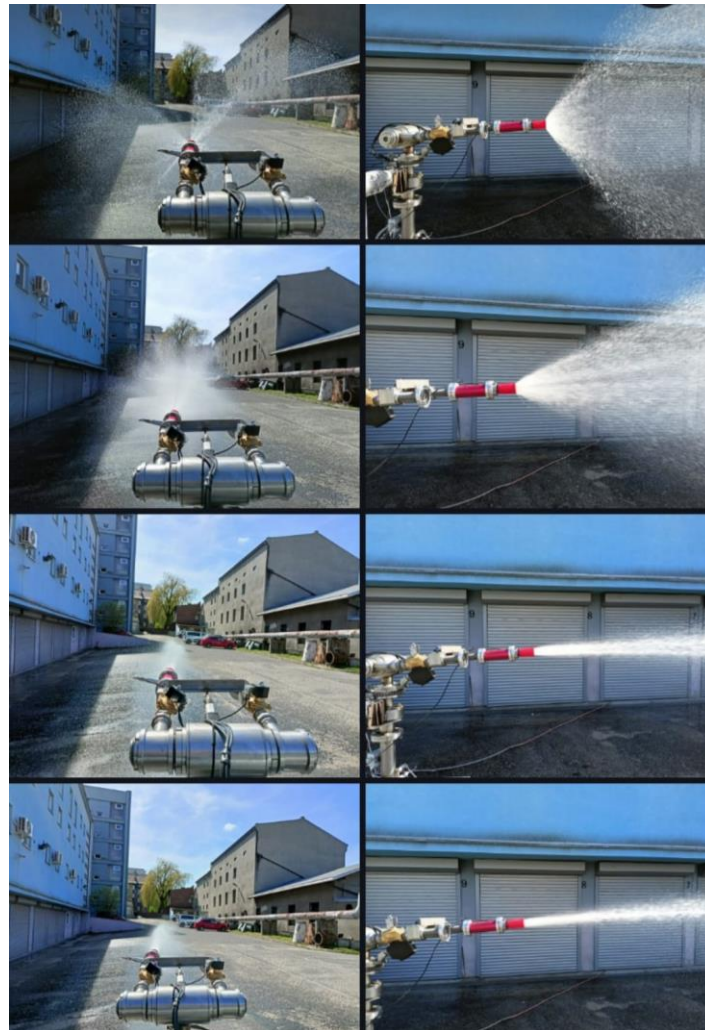
Fig. 12. Photographic documentation of the spray stream shape generated by the water spray nozzle (DW) at different outlet adjustment settings (from top: 2.0, 1.5, 1.0, and 0.5 turns of the nozzle outlet)
