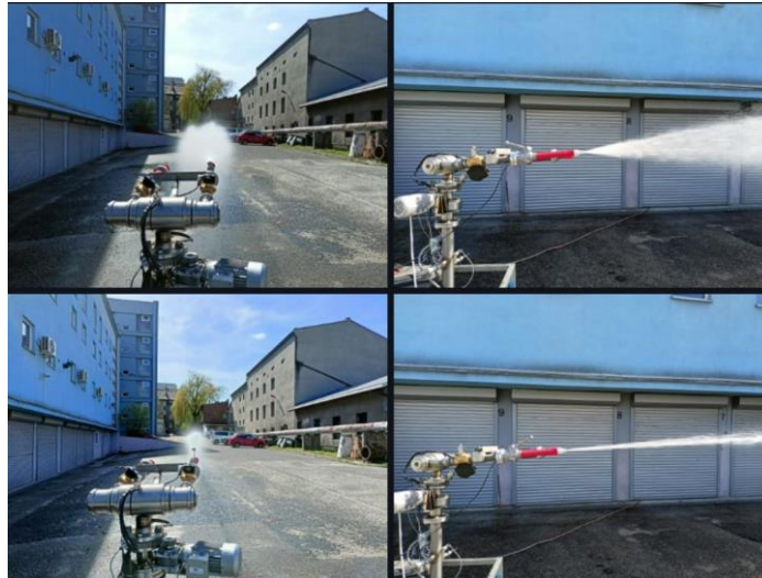
Fig. 13. Photographic documentation of the spray stream shape generated by the mulch spray nozzle (DM) at different operating positions (top: position III, bottom: position II)
