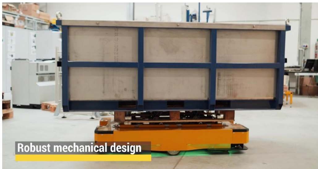
Fig. 4. AMR transporting goods larger than the outline of the trolley
