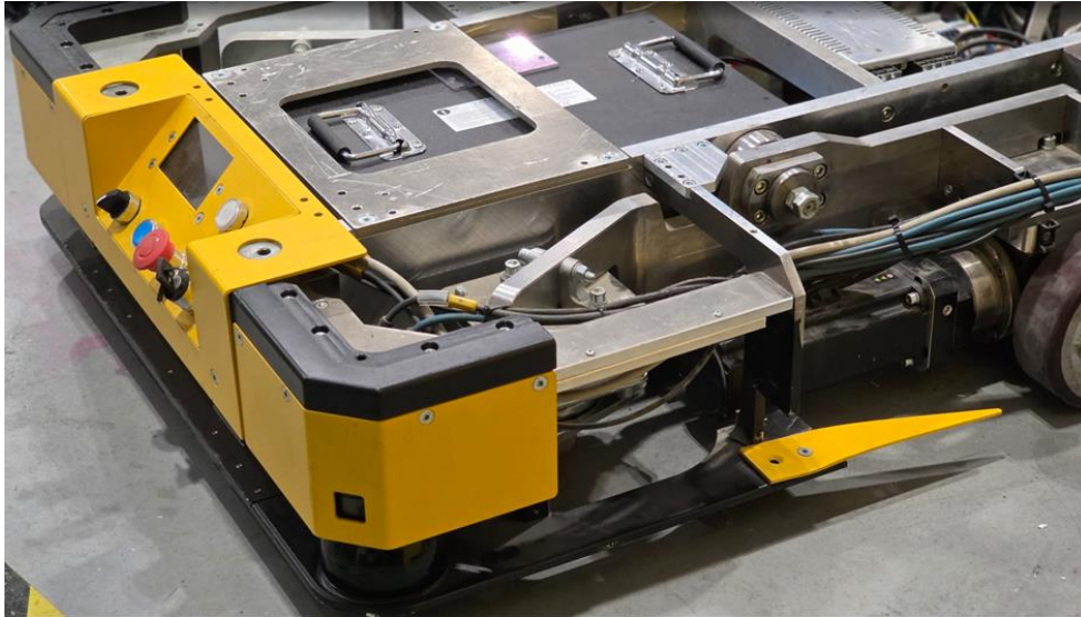
Fig. 2. Photo of the drive wheel suspension arm in the designed robot
