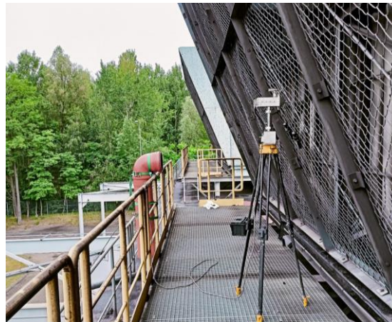
Fig. 3. Measurement station at the representative point of the Shaft VI diffuser [5]
