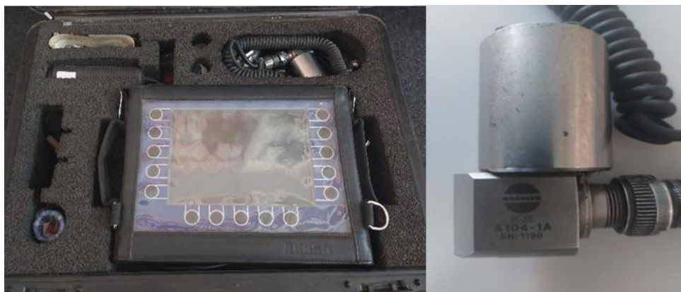
Fig. 2. ADASH A4400 VA4Pro vibration diagnostic device with A104-1A vibration sensor
