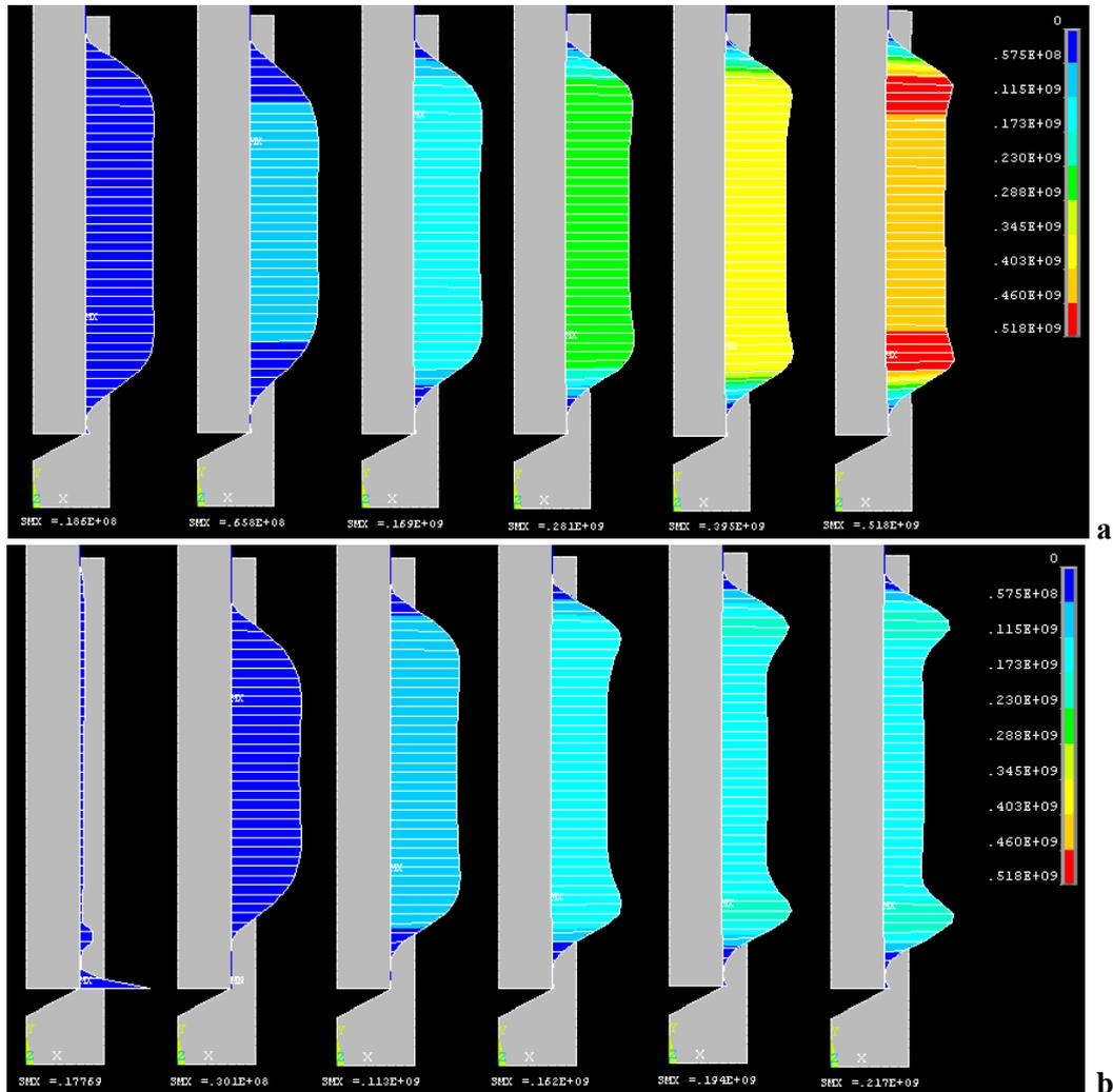
**Fig. 10.** Distribution of contact pressure along the length of the contact at the moment of compression (a) and after compression (b) at a compression pressure of 100, 200, 300, 400, 500, 600 MPa, respectively
