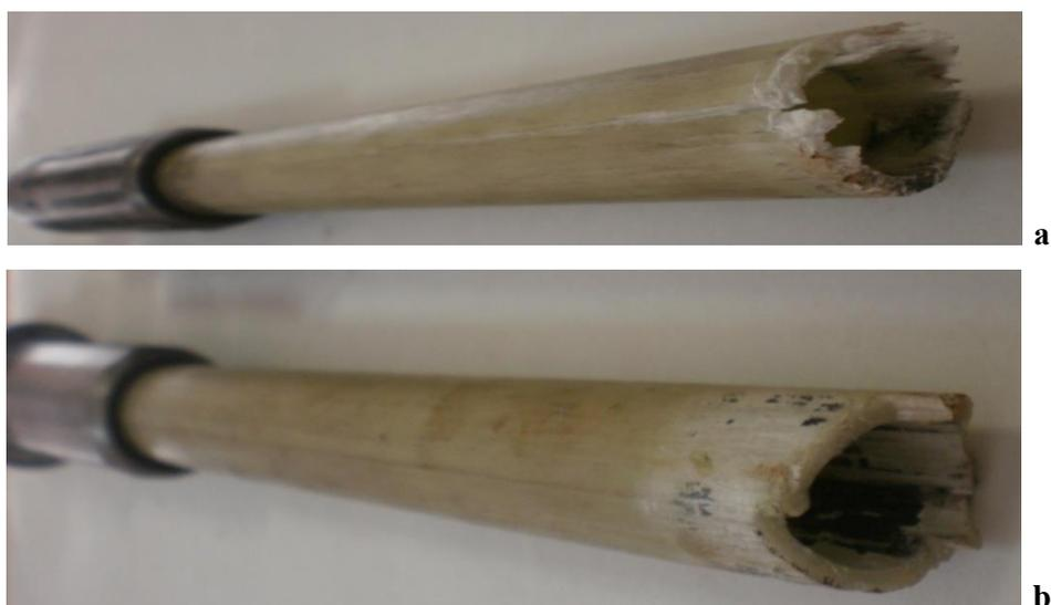
**Fig. 4.** Specimens after static tensile strength testing (a) and cyclic bending (b) Increasing the strength of the connection between the fiberglass body of the sucker rod and the steel head
