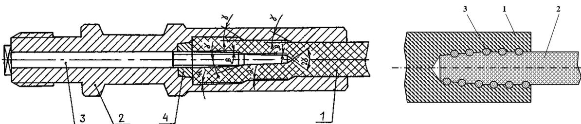
**Fig. 8.** Designs of wedge-type detachable joints (first from the left side) and with screw insert (second from the left side)
