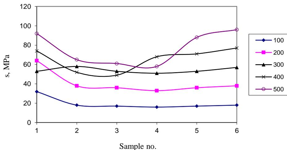
**Fig. 7.** Maximum value of contact pressure in the areas of contact of the head with the wedges at different values of external load (MPa)
