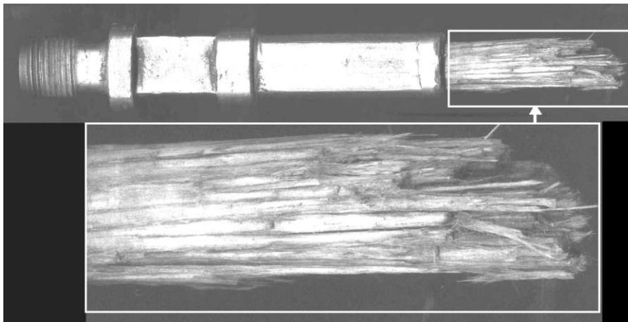
**Fig. 2.** Typical fracture of a fiberglass rod along the body
