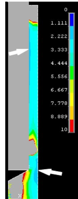
**Fig. 12.** Distribution of the fatigue safety factor  $D$  during uniform compression with a force of 400 MPa and a change in axial load from 0 to 250 MPa
