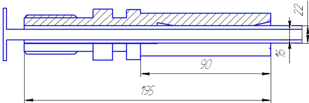
Fig. 5. Design of the sucker rod head for a wedge-adhesive joint
