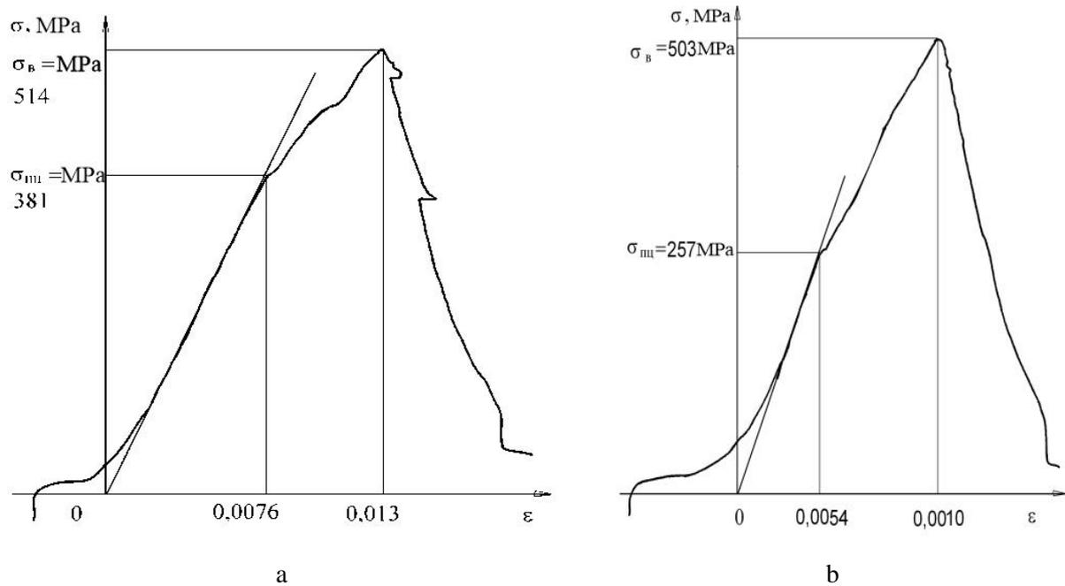
**Fig. 1.** Tensile diagram of samples of new solid fiberglass sucker rod (a) and new tubular fiberglass sucker rod (b)
