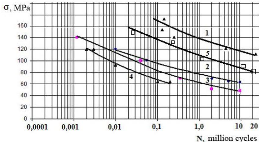
**Fig. 3.** Fatigue resistance curves of hybrid sucker rods (1), fiberglass (2-4) and carbon fiber (5) during cyclic bending: 1 - hybrid rods in mineralized formation water, 2 - hollow original design in oil with 10% HCl, 3 - reinforced design in formation water with oil, 4 - usual design in mineralized formation water, 5 - hollow carbon fiber UKN / 5000 modified by atmospheric plasma treatment with acrylic acid original design sucker rod in mineralized formation water
