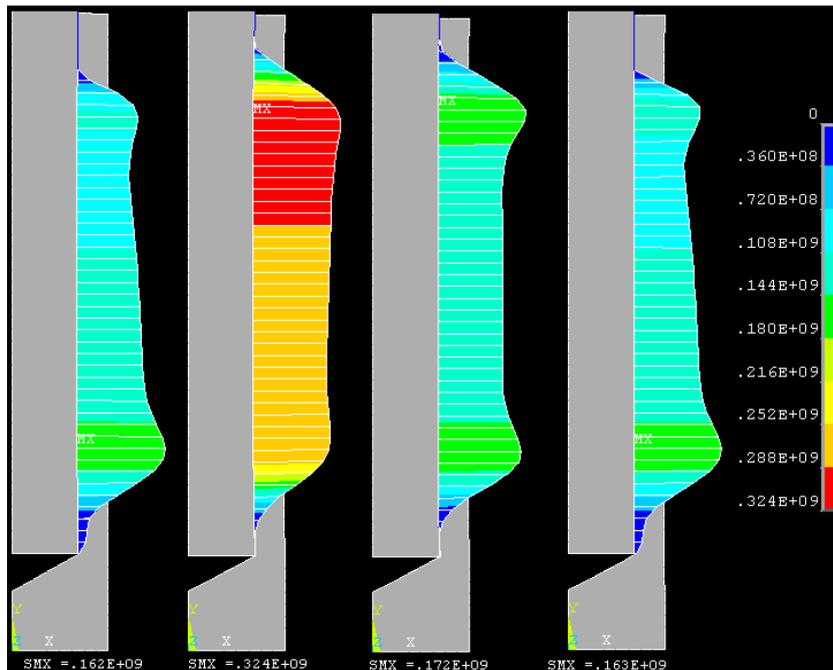
**Fig. 11.** Distribution of contact pressure along the length of contact during compression with straight (a – first from the left) and inclined (b, c, d – from the left next accordingly) dies: at the moment of compression (b), after compression (c) and at the moment of reaching a tensile load of 500 MPa (a - d)
