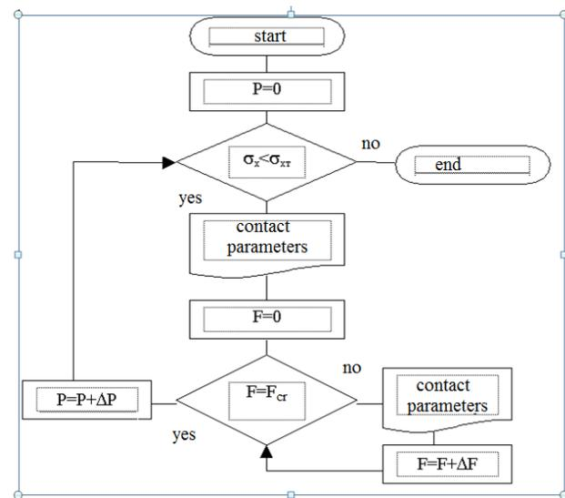
**Fig. 9.** Scheme of the algorithm for optimizing the compression force:  $P$  - compression pressure;  $\Delta P$  - step of changing the compression pressure;  $F$  - external axial load;  $\Delta F$  - step of changing the axial load;  $F_{cr}$  - critical value of the external axial load;  $\sigma_x$ ,  $\sigma_{xt}$  - stresses and yield strength in the radial direction of the fiberglass rod
