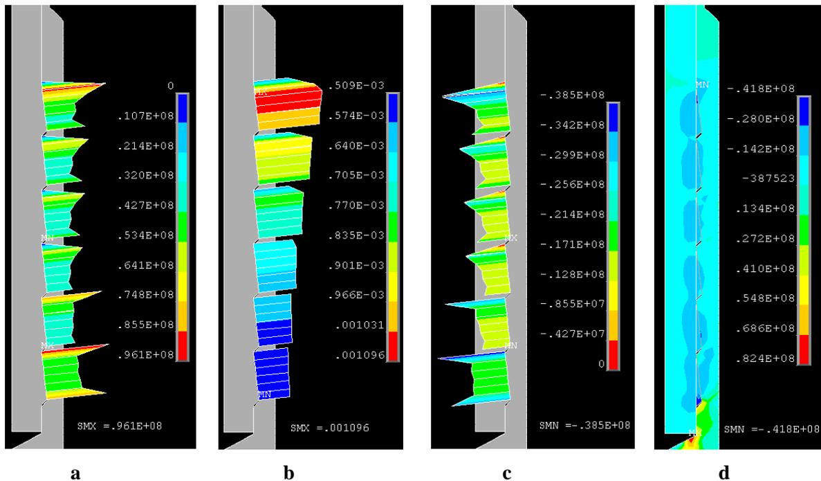
Fig. 6. Characteristics of a wedge-adhesive joint of a rod with a diameter of 22 mm at an external load of 500 MPa contact pressure, MPa (a), slip value, m (b); shear stress, MPa (c) in the area of contact of the head with the wedges;  $\tau_{xy}$ , MPa (d) distribution of tangential stresses
