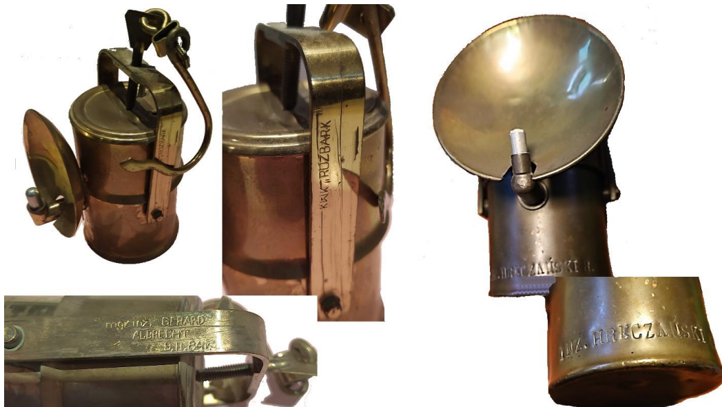
Fig. 4. Examples of personalized carbide lamps [source: own collection of authors]
