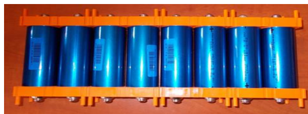
Fig. 2. The battery consists of eight lithium-iron-phosphorus cells (LiFePO 4 )
