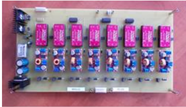
Fig. 4. Measurement and control module
