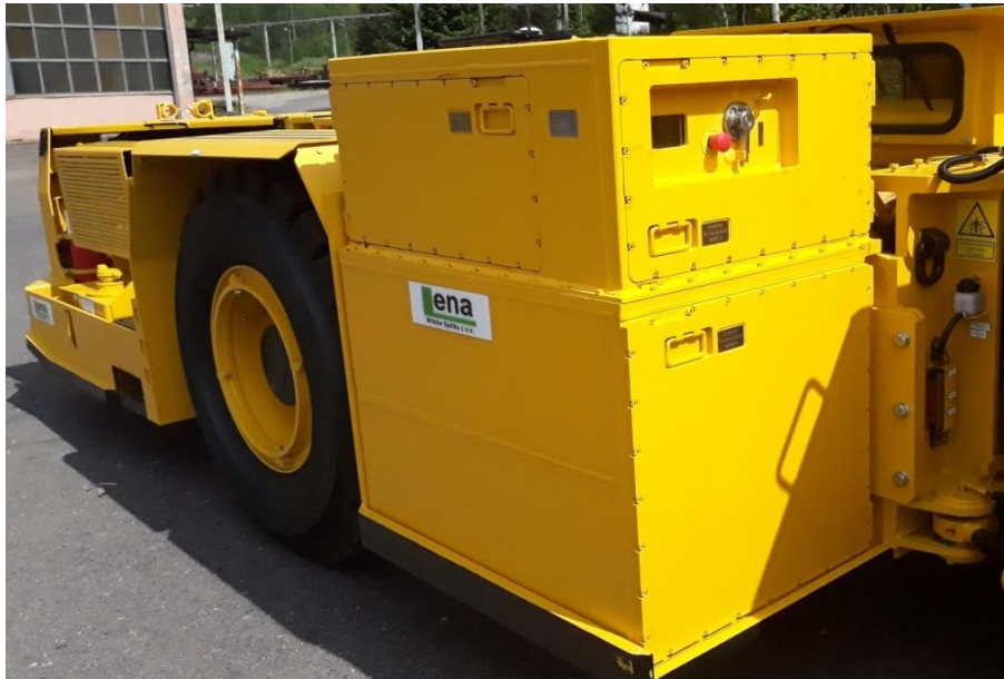
Fig. 5. ZZB battery power supply unit installed in the SWS-1700ENB blast truck
