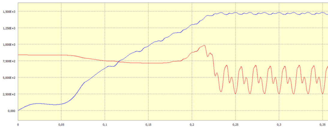
Fig. 8. Characteristics of the 45 kW 225M motor and the speed and torque waveforms for the crankshaft drill
