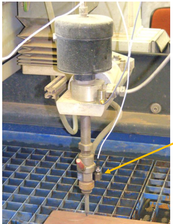
Fig. 1. Technological head with installed accelerometer marked with an arrow
