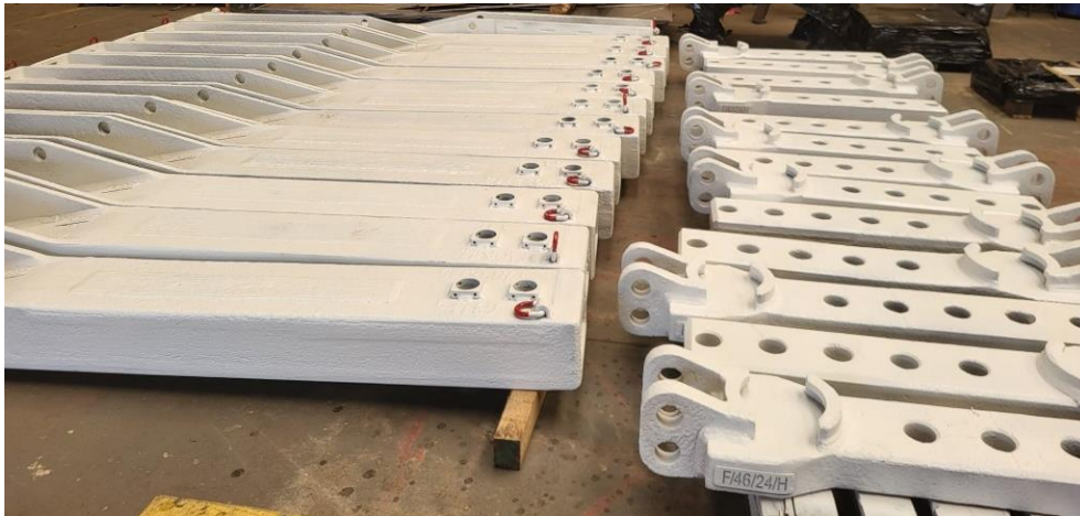
Fig. 11. Beam of advance system and bush bar after repair
