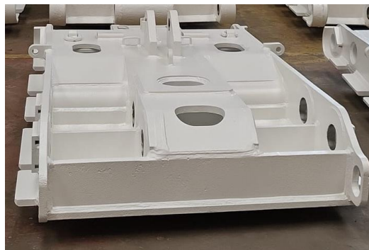
Fig. 7. The gob shield after modernization
