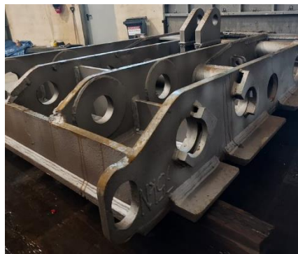
Fig. 4. The gob shield after shot blasting
