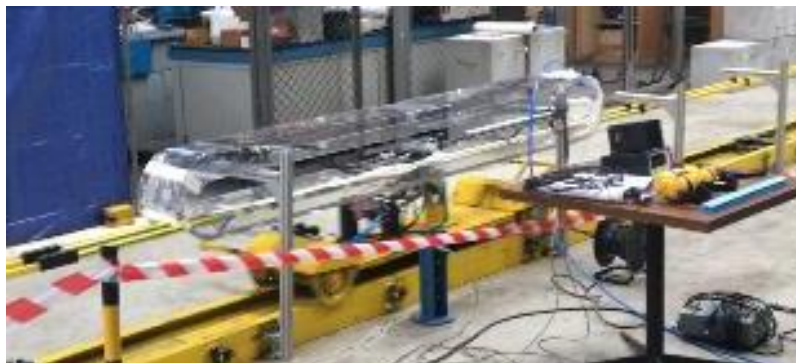
Fig. 10. View of the transparent container, two busbar lines running across, the trolley on the C-section route below [1]
