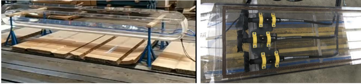
Fig. 8. The transparent two compartment container HMC (on the left), three fans with adjustable speed up to 20,000 rpm installed inside the upper HMC compartment [1]
