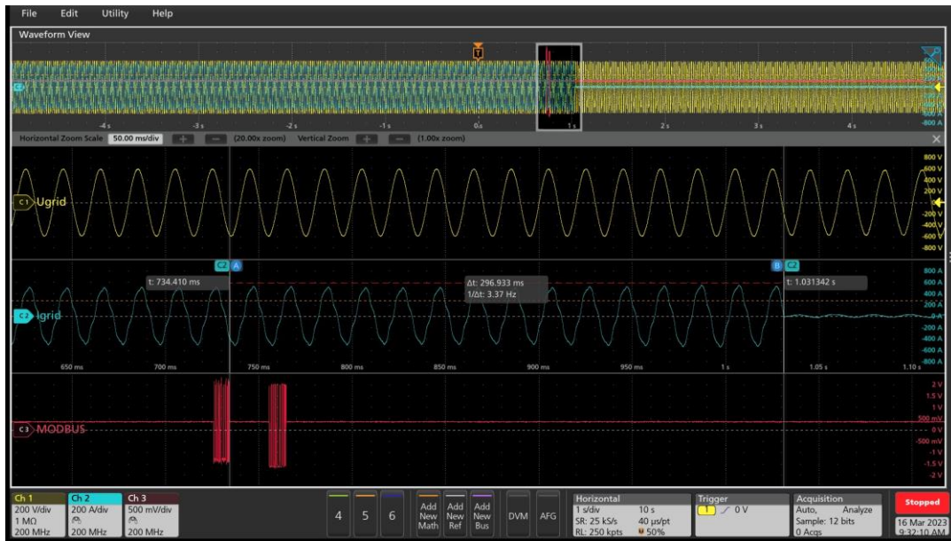
Fig. 5. A diagram illustrating the time to stop active power generation after accepting a command at the input port (logical interface)
