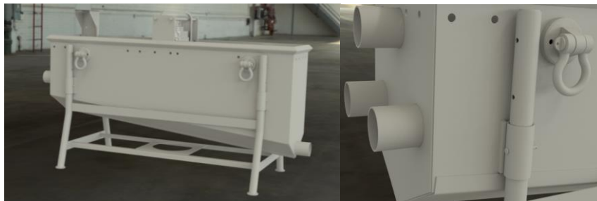
Fig. 15. Base water tank with adjustable support frame
