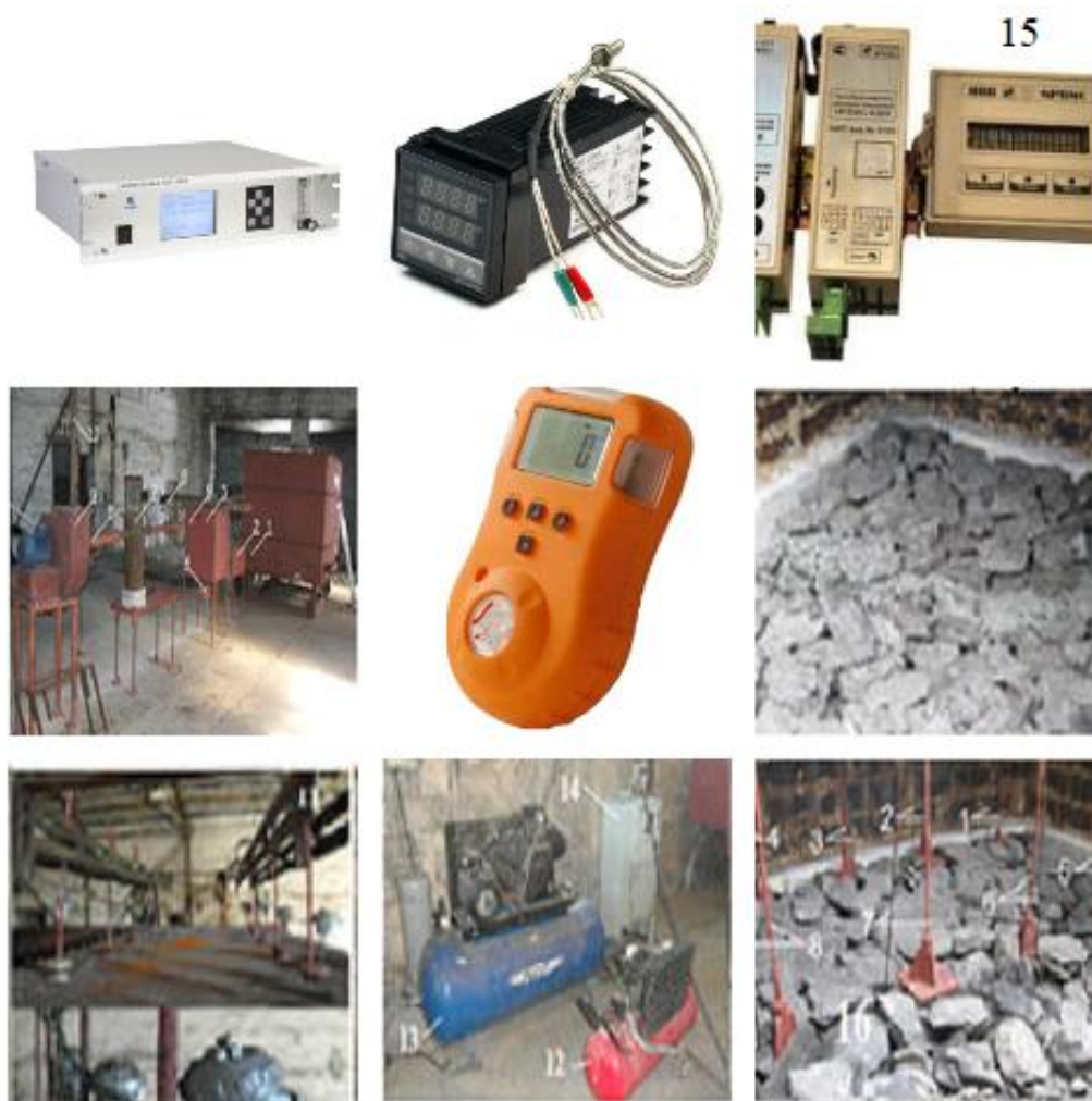
Fig. 1. Assembly, preparation and testing the SPGV in ESU: 1 – transitional cooling box; 2 – condensate tank; 3 – generator gas cooling tank; 4 – a container for collecting condensate; 5 – gas outlet pipeline; 6 – IRVIS sensor; 7 – configurator for cleaning generator gas from hydrogen sulphide (H 2 S); 8 – chimney; 9 – transition pipe; 10 – vertical gas outlet pipe; 11 – section No. 1, testing and measuring complex (thermocouples): display of temperature sensors (thermocouples), TERA "Devices System" software based on the Firebird 2.1 database; 12 – reserve compressor; 13 – main compressor; 14 – steam generator; 15 – section No. 2, system for controlling quantitative parameters of generator gas blowing and pressure: IRVIS - K300, gas analysers Garboards 3200L and BX-170. The change in displacement of the roof rocks, as the gasification area of the gas generator increases, was provided by the database of reference sensors and the Monitor QB program; 16 – formation of a solid coal together with the installation of reference sensors
