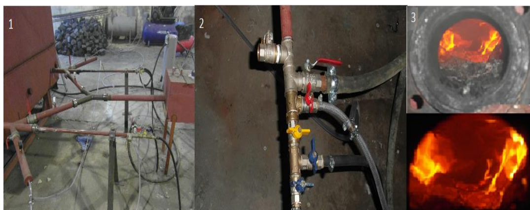
Fig. 2. The coal seam ignition process and the thermal treatment of the reaction channel of the underground gas generator model: 1 – connection of the unit for the integration of the supply and discharge of blast mixtures and generator gas with the gas generator stand; 2 – the control system for blast supply modes and reverse operations; 3 – visualization of the activation of oxidation and reduction zones when applying reverse streams
