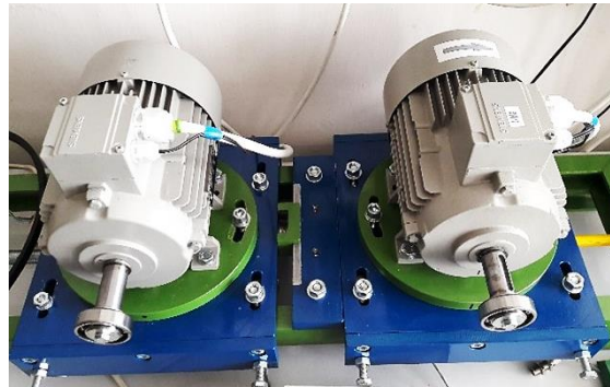
Fig. 2. Test bearings mounted on the experimental stand
