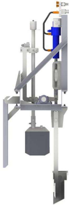
Fig. 4. Slide-gate discharge system [19]
