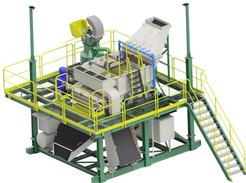
Fig. 11. Prototype of the mobile mining waste separation system S-100 [26]
