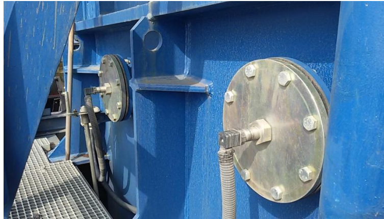
Fig. 10. Pressure sensor installed in the air chambers of the working compartment [16]
